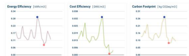
Figure 2. Key performance indicators for energy, cost efficiency and carbon footprint at Egå WRRF. Presented trends are based on real-time simulations (21:00, 06/04/2022) with hindcast period of 48 h.
