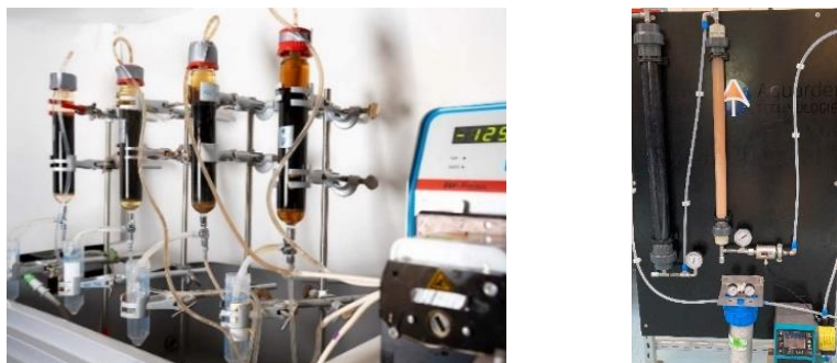
Figure 1: Column-setup for adsorption efficiency evaluation of various leachate waters. Left: Laboratory setup 100-mL columns and right: small-scale side-stream field-setup (250mL columns).
