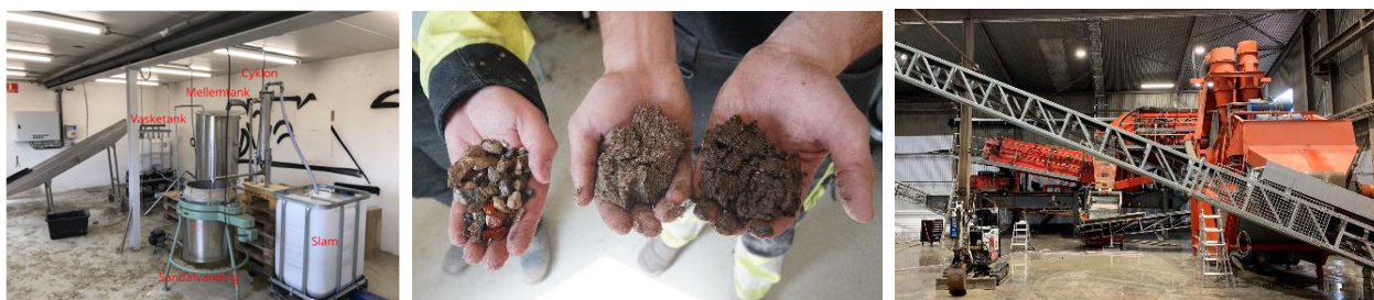
Pilot scale soil washer (left), washed stones, sand, and unwashed soil (middle), full scale soil washer (right)
