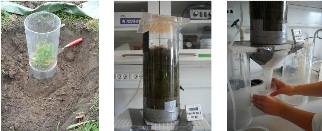
Figure 1. The treatment efficiency of an intact soil column from a German swale-trench is tested in the laboratory.
